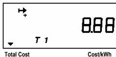
Fig.: 2.3 / 3.3 Total Cost T1 / T2 (Total Cost) 0.00 - 99999.99 Total Cost Overflow: Stop at 99999.99 Total Cost
