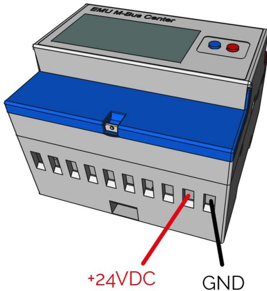
The M-Bus Center needs a 24VDC supply voltage with a current of at least 1A.
